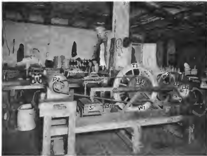
Fig. 13—Tire-testing machine as used in the Woods plant at Chicago for testing out tires
